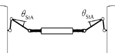
The angle that is actually important, the deviation from 90at the steering arm to track rod joint
