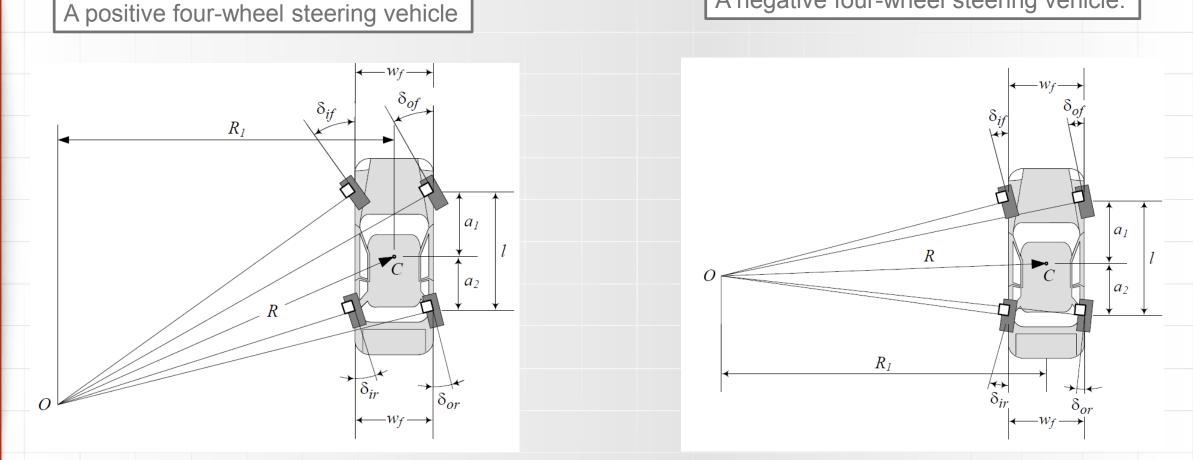
In a **positive** 4W S situation the front and rear wheels steer in the same direction, and in a **negative** 4W S situation the front and rear wheels steer opposite to each other
