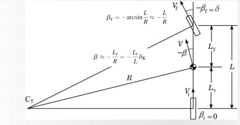
Attitude angle is positive with the vehicle pointing towards the inside of the corner, so the angles are negative in the figure
