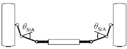
**Inclination of the steering arms is not required at all**, it can all be done by positioning the rack to give the necessary included angle. With this method, forward steering arms need not be angled out, and can even be angled inwards. although this increases the loads and wear on the rack
