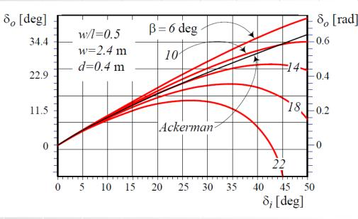
For a given I and w, a mechanism with  $\beta \approx 10$  deg is the best simulator of an Ackerman mechanism
