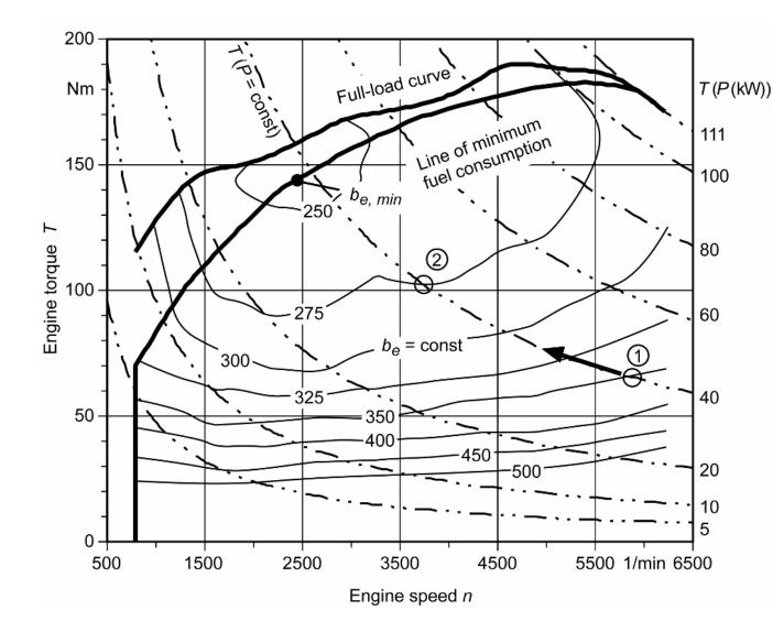
A minimum fuel consumption point can be found on any power hyperbola. The curve passing through these points is the minimum fuel consumption curve.
