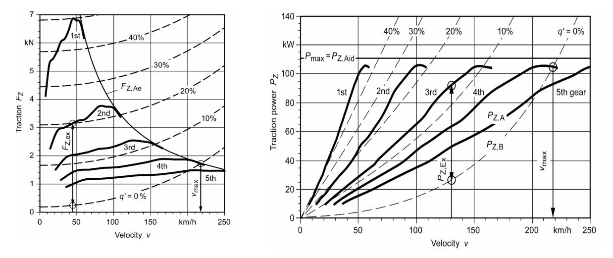
The maximum speed, the maximum climbing performance and excess traction in the various gears can be found from the traction diagram.
