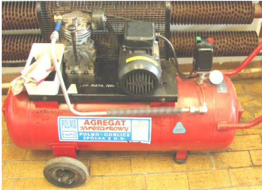
Fig 1 Compressor installation as a measurement position
