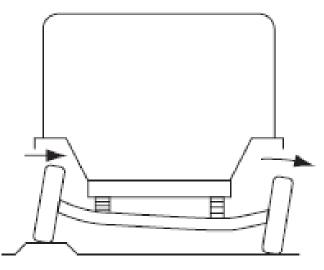
Both wheels tilt when either passes over an obstacle
