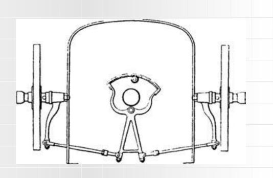
Ackermann steering effect achieved with parallel steering arms, by using angled drive points at the inner end of the track rods: 'La Mancelle', 1878.
