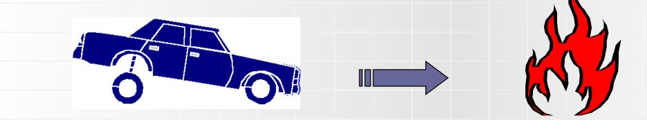
The brake system converts the kinetic energy of vehicle motion into heat
