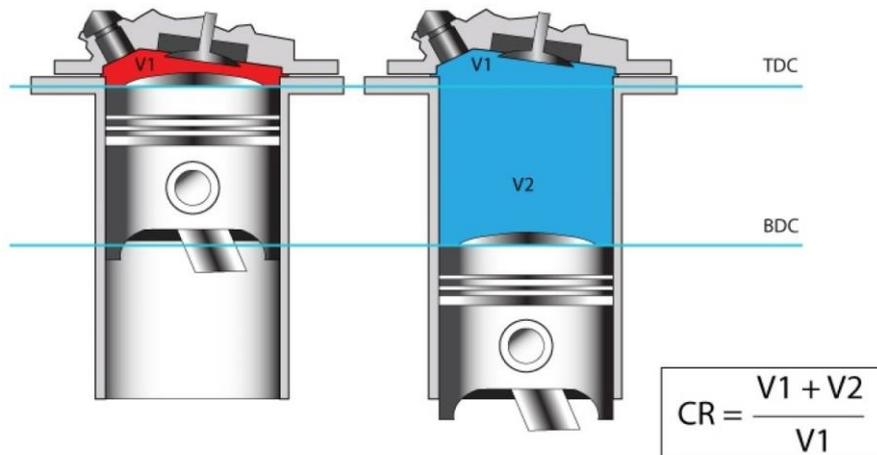
**Compression ratio** – the ratio of the maximum volume in cylinder at piston BDC to the volume in cylinder at piston TDC
