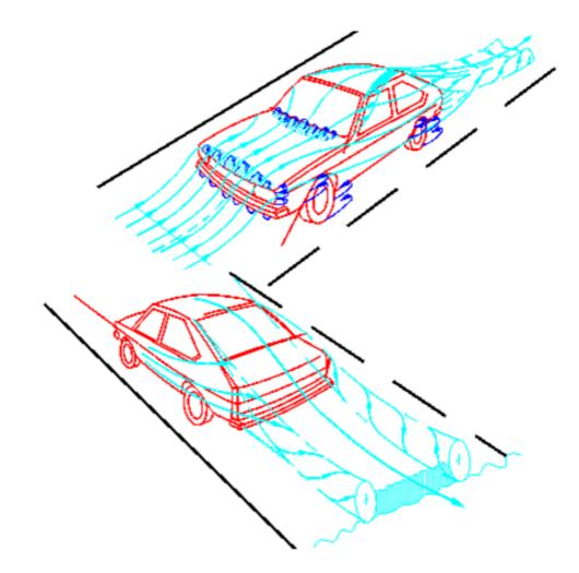
Faster airstream low pressure over upper body surface Ideal aerofoil car shape Air moving from low to high pressure region Direction Trailing vortex cone of motion Merging airstream Slower airstream and higher air pressure-underneath body (a) Pictorial view Trailing vortex Liagonal airstream cone Negative ( =pressure Direction of motion
