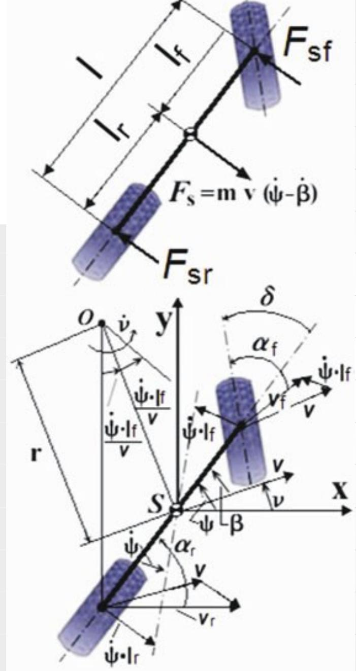
To negotiate a circular path according to Olley's definition, the driver must input a larger steering angle for a vehicle with understeer than for a vehicle with neutral handling characteristics
