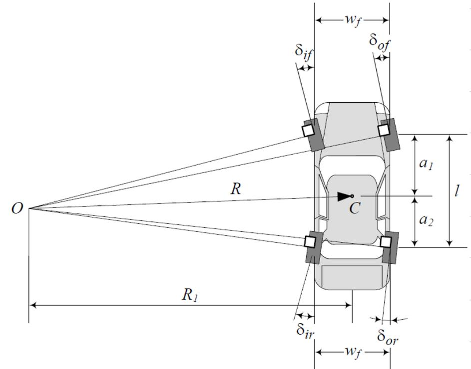
In a **positive** 4W S situation the front and rear wheels steer in the same direction, and in a **negative** 4W S situation the front and rear wheels steer opposite to each other
