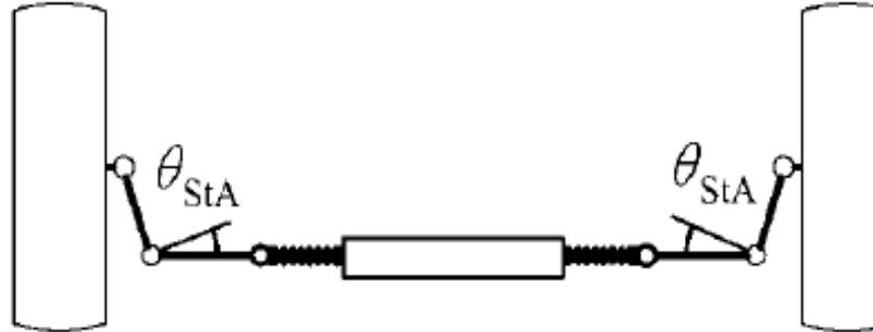
Angle opened up by moving the rack to the rear, increasing the Ackermann effect
