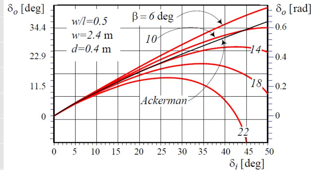
For a given  $l$  and  $w$ , a mechanism with  $\beta \approx 10$  deg is the best simulator of an Ackerman mechanism
