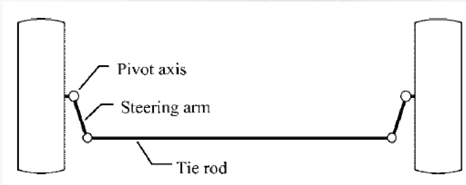
The steering arm angle usually considered important, as indeed it is with the aligned rack and track rods
