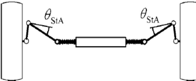
Considering the included angle between the track rod and the steering arm, with a conventional system, the steering linkage Ackermann effect angle, ideal (100%) Ackermann requires
