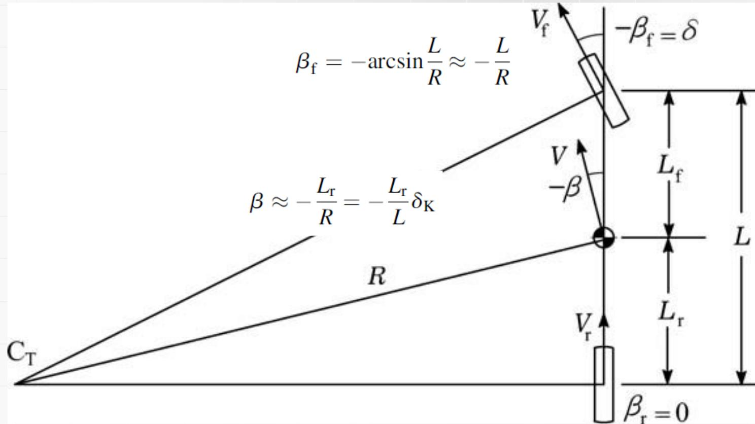
*Attitude angle is positive with the vehicle pointing towards the inside of the corner, so the angles are negative in the figure*
