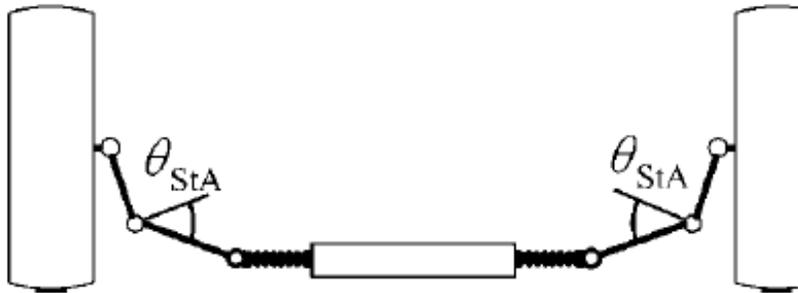
**Inclination of the steering arms is not required at all**, it can all be done by positioning the rack to give the necessary included angle. With this method, forward steering arms need not be angled out, and can even be angled inwards. although this increases the loads and wear on the rack
