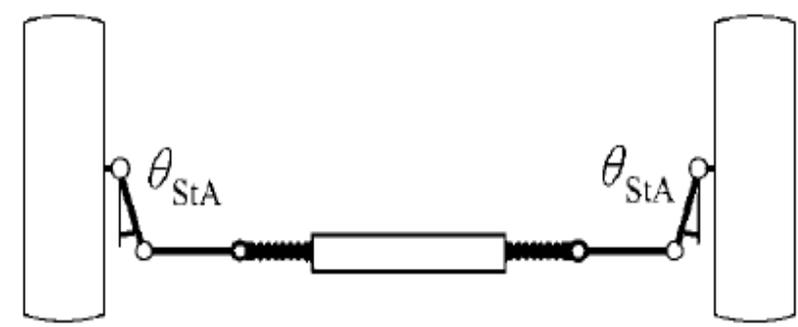
The angle that is actually important, the deviation from 90 at the steering arm to track rod joint
